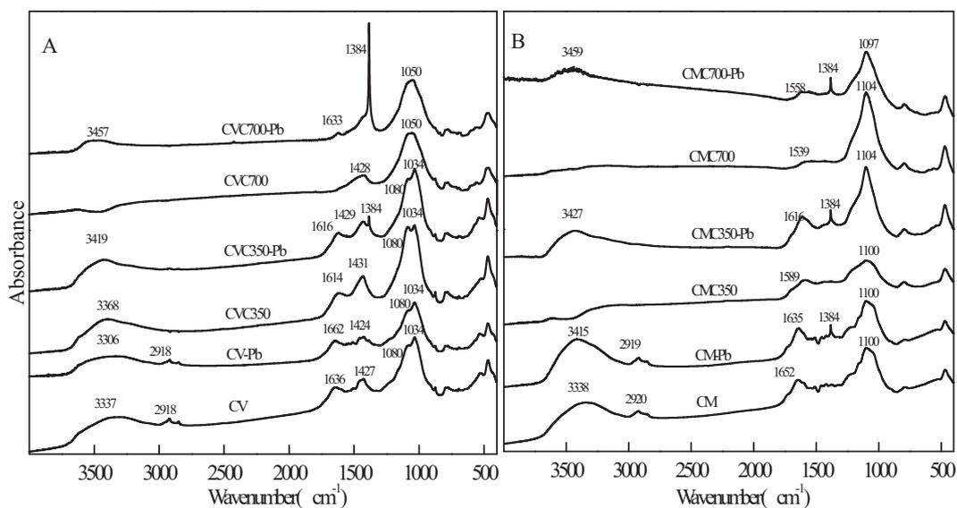
Fig. 5. Stacked FTIR spectra of the adsorbents before and after  $Pb^{2+}$  adsorption.
