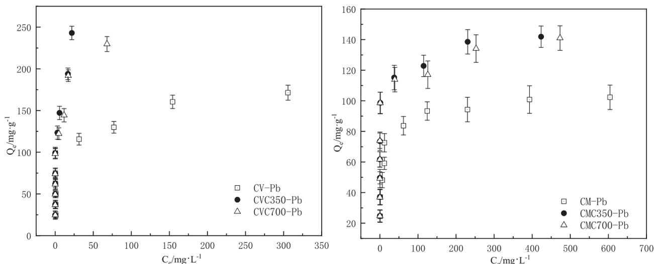
**Fig. 2.** Adsorption isotherm curve of  $\text{Pb}^{2+}$  onto CV, CVC350, and CVC700 and CM, CMC350, and CMC700.
