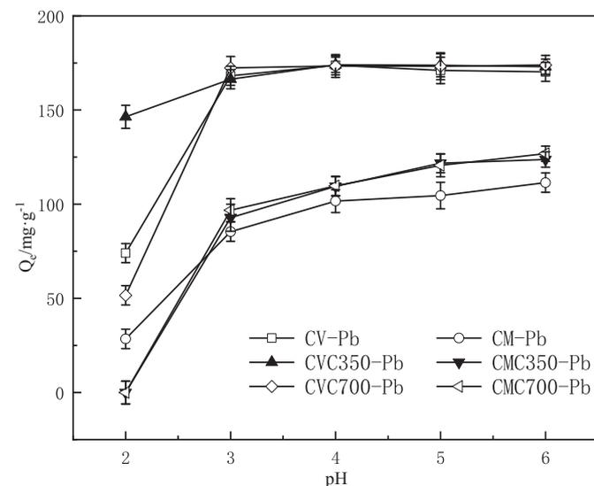
**Fig. 3.** Effect of initial solution pH on  $Pb^{2+}$  adsorption.
