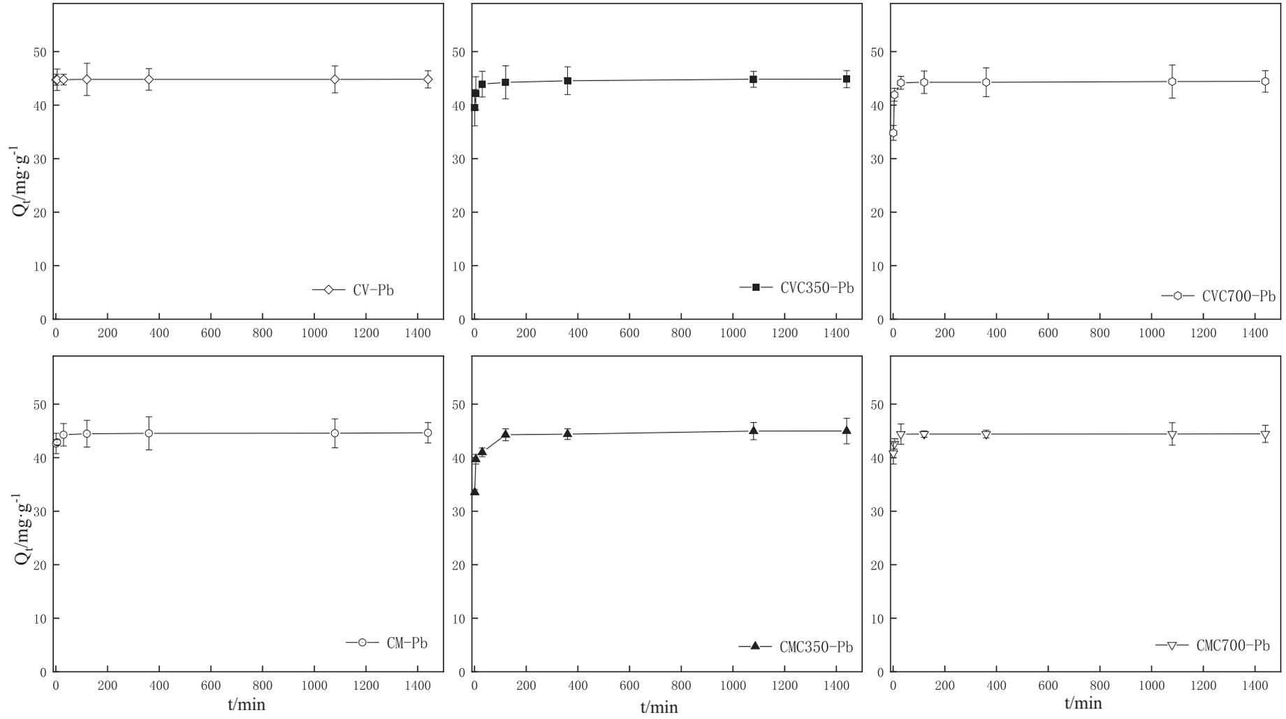
Fig. 4. Kinetics of Pb<sup>2+</sup> adsorption by CV, CVC350, and CVC700 and CM, CMC350, and CMC700.
