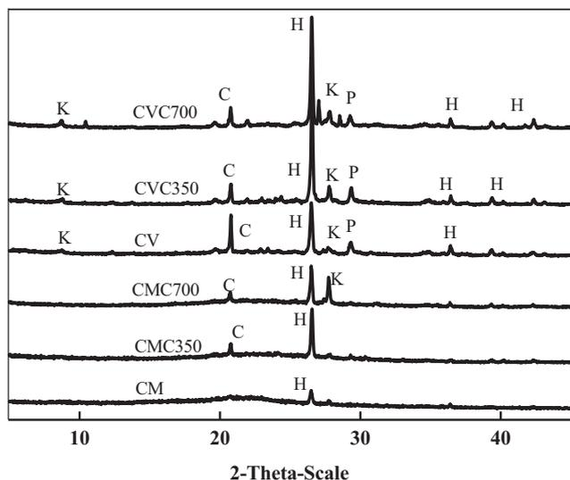
**Fig. 1.** X-ray diffraction patterns of CV, CVC350, and CVC700 and CM, CMC350, and CMC700 material minerals, with peaks labelled: K, kalicinite ( $\text{KHCO}_3$ ); C, quartz ( $\text{SiO}_2$ ); H, halite ( $\text{NaCl}$ ); P,  $\text{CaCO}_3$ .
